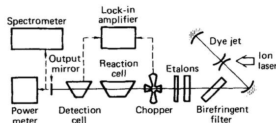
FIG. 1. Experimental layout for intracavity excitation of addition reactions. Reactants are in the reaction cell. The CW dye laser is tuned on resonance by optoacoustic detection with the detection cell. Laser power and wavelength are monitored by an external power meter and spectrometer, respectively.
